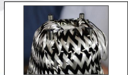
(Above: example of loose tie off of braid to facilitate full fabric saturation)
